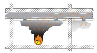
Spread of fire and smoke through ventilation ducting
