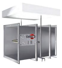
The fire dampers are suspended using threaded rods. The rods can be bare if their length does not exceed 1.50 m; longer rods require insulation.
