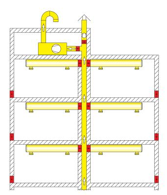
Ventilation with a combined ventilation/smoke extract system
