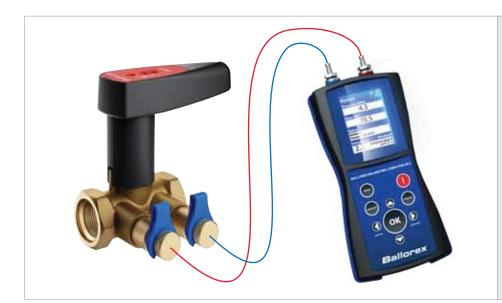
When measuring flow on a Ballorex Vario the setting is typed into the flowmeter. Every time the setting is changed, it must be re-entered in order to achieve the correct flow reading.
