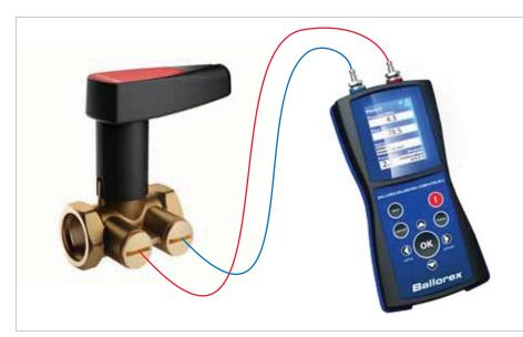
When measuring flow on a Ballorex Basic the correct type and size of the valve is first chosen from the display list. The pre-programmed Kvm-value is then used to convert the differential pressure measurement into a direct flow reading. The valve can be used for measuring only in a fully open position and with measuring points provided as accessories.
