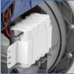
Variant with battery pack
